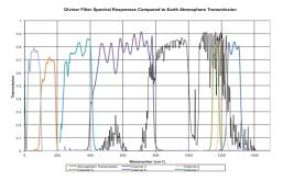
**Figure 1.** Diviner filter bandpass compared with the Earth's atmospheric transmission to space.
