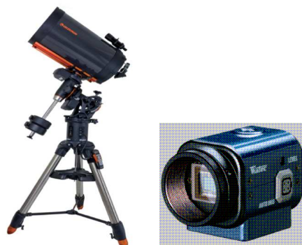
Figure 1: C14 telescope and Watec camera used for Impact Flashes Monitoring
