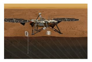
Figure 1: Conceptual view of the GEMS lander including the deployed seismometer and heat flow probe  $(HP^3)$ .
