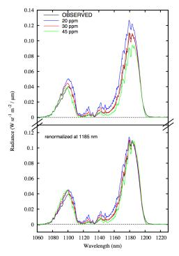
Figure 1: The SPICAV spectrum is compared to synthetic spectra calculated with H<sub>2</sub>O mole fractions of 20, 30 and 45 ppm using our best estimate for the representation of the H<sub>2</sub>O/HDO and CO<sub>2</sub> opacity. *Upper panel*: raw calculations; *Lower panel*: spectra renormalized to the observed radiance at 1185 nm.
