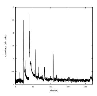
Figure 1: A sum spectrum of 32 impact ionisation mass spectra of anorthite grains which impacted at velocities of between 5 and 6 km s<sup>-1</sup> onto the LAMA laboratory model.
