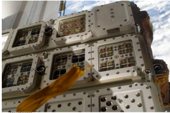
Figure 1: The EXPOSE-R facility outside the ISS with accommodated SPORES samples
