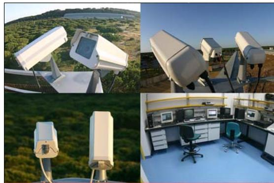
**Figure 1.** Images of the control room and some of the high sensitivity CCD video cameras of the CIECEM meteor observing station.
