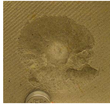
Figure 1: Experimental crater in sandstone target. Image is ~8 cm wide.
