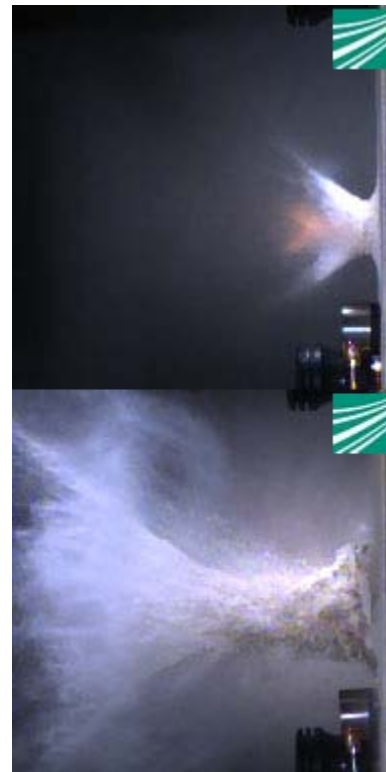
Figure 2: Two stages of the ejecta process imaged at 20 and 1000 \mu s after impact.
