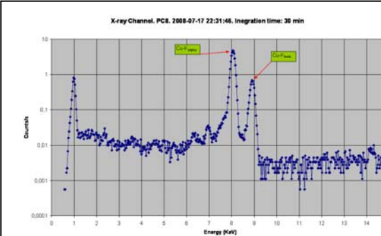
Figure 2: X-ray spectrum of the inner side of the copper doors of the APXS instrument. Lower threshold at about 1.0 keV; upper threshold at about 14.8 keV.
