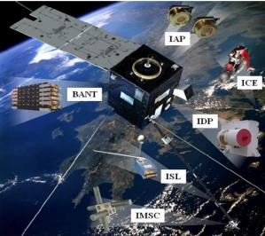
Figure 1: The schematic view of the DEMETER satellite and its instrumentation.
