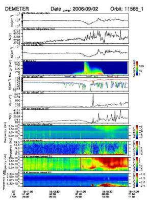
Fig.3 Plasma parameters and ELF plasma turbulence registered by DEMETER In the ionospheric trough.
