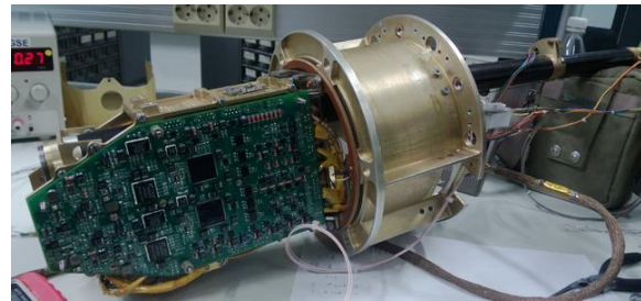
Figure 4: MetNet payload bay QM.
