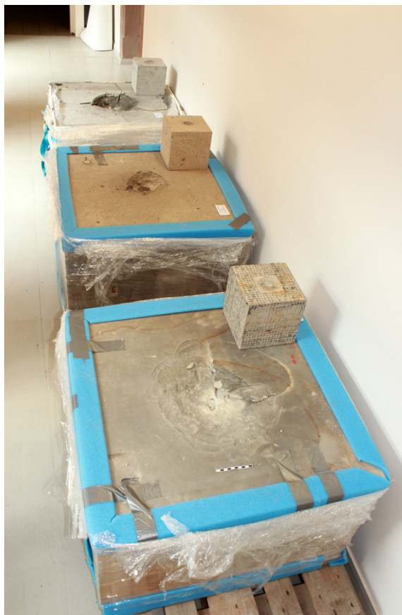
Fig. 1: Craters formed in quartzite, tuff and sandstone targets (back to front). Large targets are 80 cm wide, small targets are 20 cm cubes.
