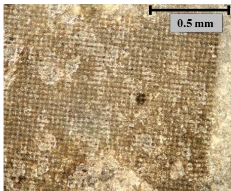
Figure 2: Measurement locations on the Allende meteorite with a spacing of 30\ \mu\text{m} between laser spots. Four measurement points are situated on a dark inclusion.
