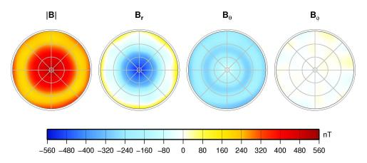
Figure 1: Stereographic north polar view maps of the predicted magnetic field from first solar day MESSENGER measurements. Maps are obtained at 200 km altitude, in Mercury body fixed coordinates. Grid lines are every 45° for longitude and every 30° for latitude. From left to right: Intensity, radial, co-latitudinal and longitudinal field components.
