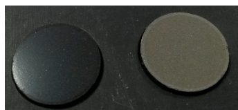
Figure 4: Pellets (13mm in diameter) of CM Mighei (left) and CO Lencé (right). On the edge of the pellet, one can see an unirradiated area (corona of 500 \mu\text{m} ): the altered region gets darker for the CO and brighter for the CM.
