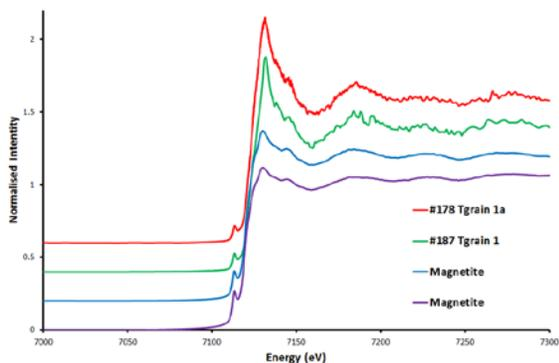
Fig. 3: Fe-K XANES plots of Track #178, #187 terminal grains compared to a powdered magnetite standard.
