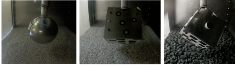
Figure 1: The two projectiles used in the experiment. Left: spherical projectile in an experiment with quartz sand. Middle: cubic projectile positioned to impact the quartz sand on the projectile edge. Right: cubic projectile positioned to impact the basalt gravel on the projectile corner.
