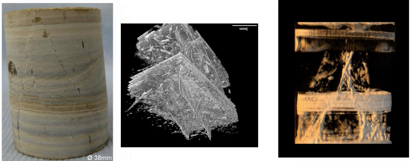
**Figure1.** Figure shows (a) deformed laminite cylinder 38mm in diameter with observable and apparently dominantly open vertical and steeply inclined fractures; (b) x-ray tomography of a central section of the deformed laminite cylinder; and (c) neutron tomography of the whole sample when liquid was approaching the top surface.
