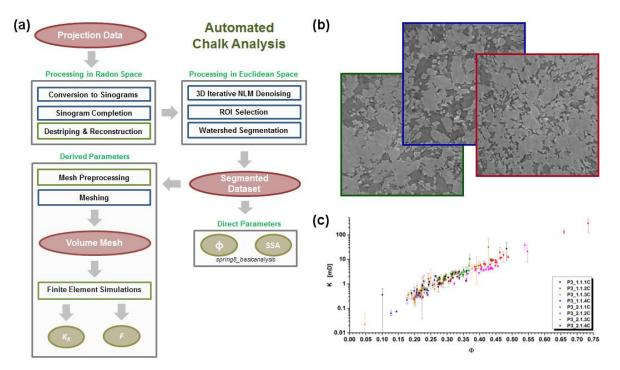
**Figure 1:** (a) Outline of the operations performed during the automated tomography image processing. (b) Examples of 2D slices after 3D iterative denoising and (c) the final results shown for the porosity-permeability.
