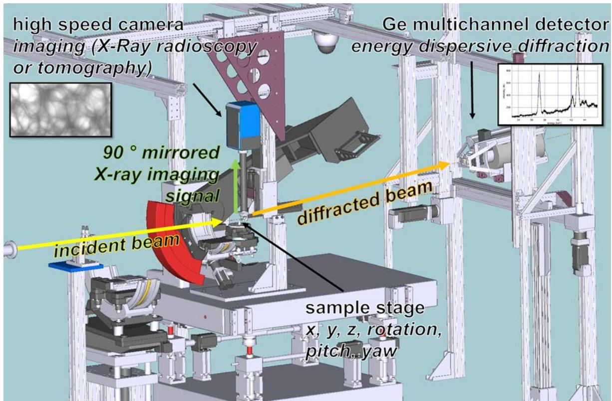
**Figure 1:** Overview of the instrumentation at the EDDI beamline, Bessy II, Berlin. The setup for simultaneous X-ray radioscopy/tomography with energy dispersive diffraction is composed mainly of a diffractometer and a high speed camera. The yellow line depicts the incident, the green one the transmitted and the orange one the diffracted beam. The insets show a radiography of a liquid metallic foam (left) and the corresponding diffraction pattern (right).
