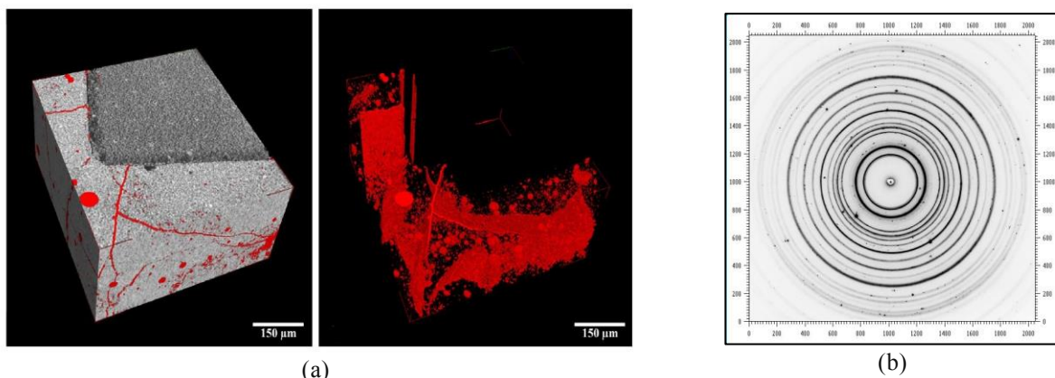
Figure 1: Mortar bar affected by ASR: (a) rendering of the weathered samples with microcracks surrounding the aggregates (X-ray tomography); (b) diffraction image collected during X-ray diffraction tomography experiments.
