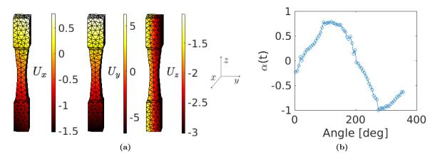
Figure 1: 3D displacement field for the first rigid body mode (a) in the x,y and z direction expressed in voxels (1 vox $\rightarrow$ 2.8  $\mu$ m for a 900 vox length specimen) associated to the temporal amplitude  $\alpha(t)$  (b). This displacement corresponds to a vertical translation and a rotation along the x direction. It can be noted that  $\alpha(t)$  that results from independent computations for each step is not much noisy hence is an accurate amplitude of the identified displacement
