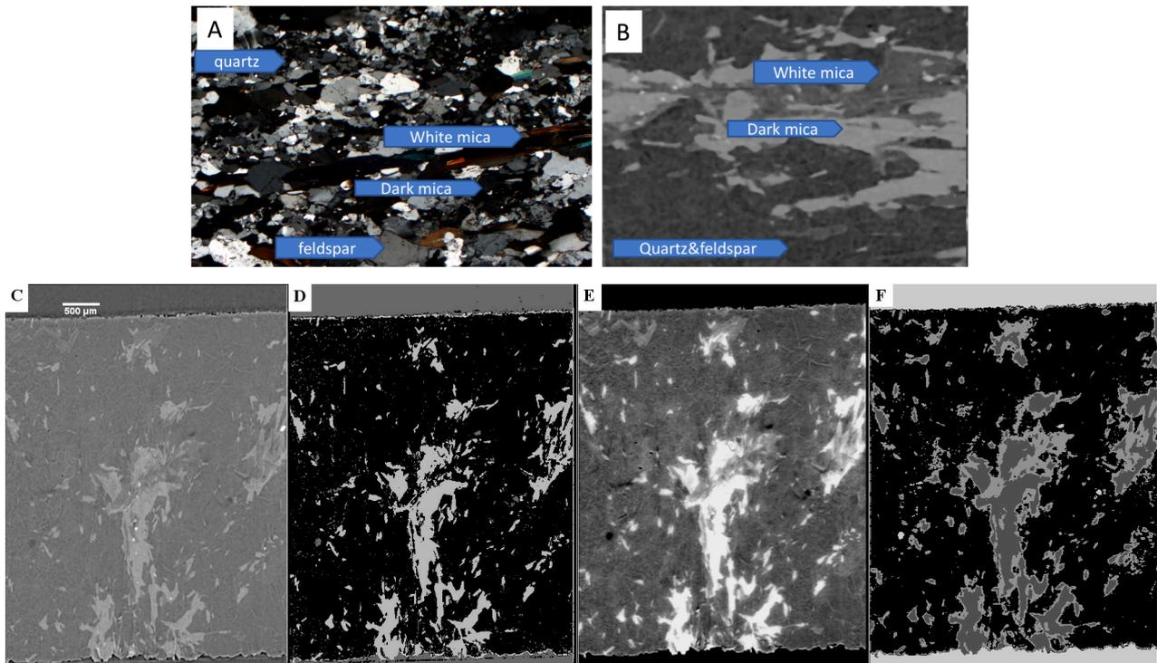
**Figure 1.** A) Optical and B) SEM images of the mylonitic metagranite (long side of the photograph = 1 mm). A sagittal section of the sample investigated by synchrotron X-ray microtomography (isotropic voxel size = 9 µm): C) as reconstructed, D) k-means clustering segmentation of the image reported in C, E) after phase-retrieval and F) k-means clustering segmentation of the image reported in E).
