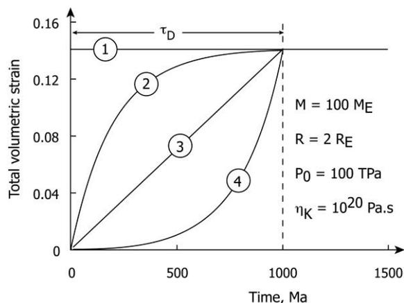
**Figure 1:** The temporal evolution of the cumulated volumetric strain induced by atmospheric unloading of a (100 Earth's mass, 2 Earth's radius) planet. Labels 1 to 4 refer to the four atmospheric loss scenarii described in the text.
