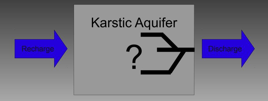
Conduits largely determine the flow and transport through the system, but in most cases we have incomplete information about the conduit network.
