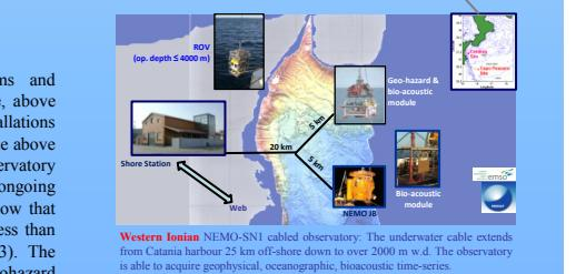
Western Ionian NEMO-SNI cabled observatory: The underwater cable extends from Catania harbour 25 km off-shore down to over 2000 m w.d. The observatory is able to acquire geophysical, oceanographic, bioacoustic time-series.
