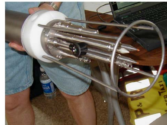
Figure 5: Sensor head of the MSS profiler. The microstructure sensors are standing in front of the other sensors. This arrangement guarantees undisturbed measurements of the micro-scale stratification and velocity fluctuations.
