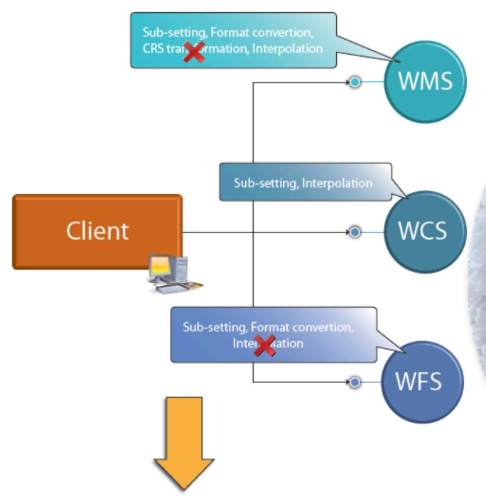
GI-axe is a distributed, a Web-based information system for improved geospatial (including sensor) data processing.
