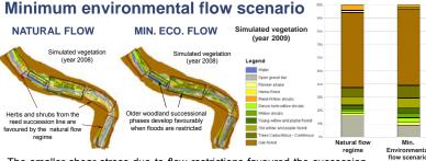
The smaller shear stress due to flow restrictions favoured the succession progress → reduced areas of open gravel bars and pioneer zones
