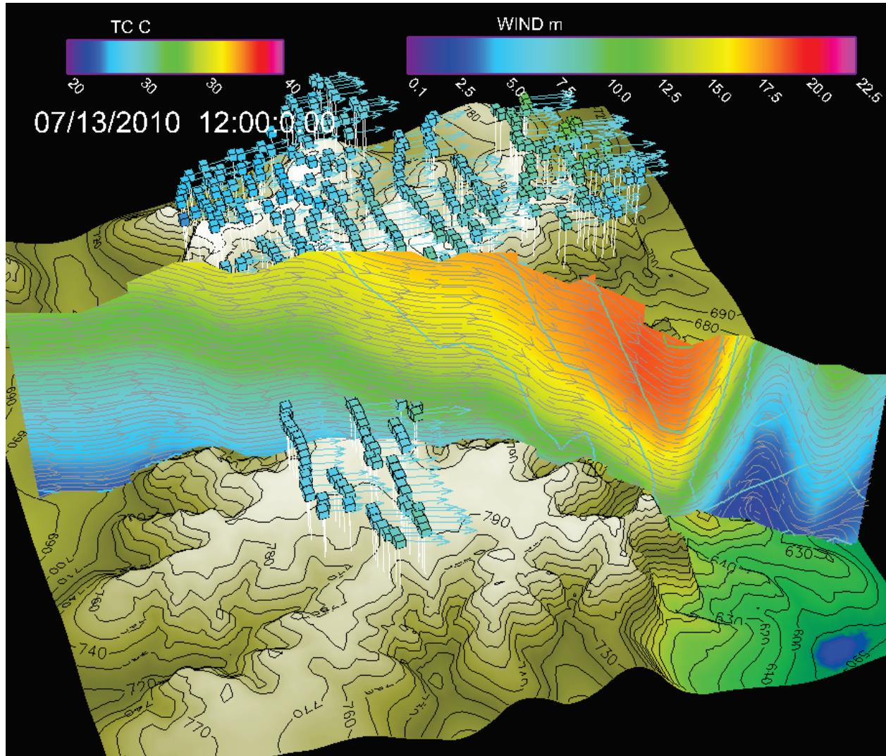
Wind turbine data compared to WRF model cross section.
