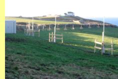
**Figure 2:** Photo of the receive antenna near Pendeen Light House on the western extent of Cornwall. Sixteen individual antenna elements are visible as well as the lab for the system electronics.
