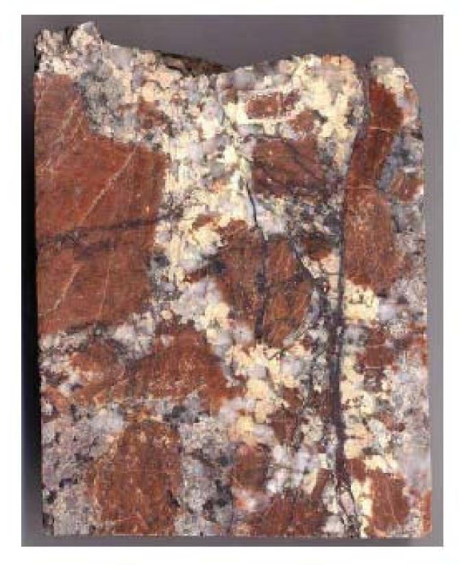
Fig. 3: Fractures in altered granite from a core taken at the EGS at Soultz-sous-Forret (Genter et al., 2009). Results from Soultz indicate that hydraulic stimulation enhanced permeability by opening previously closed weakness zones and fractures, not by creating a new network of mode-I hydraulic fractures.
