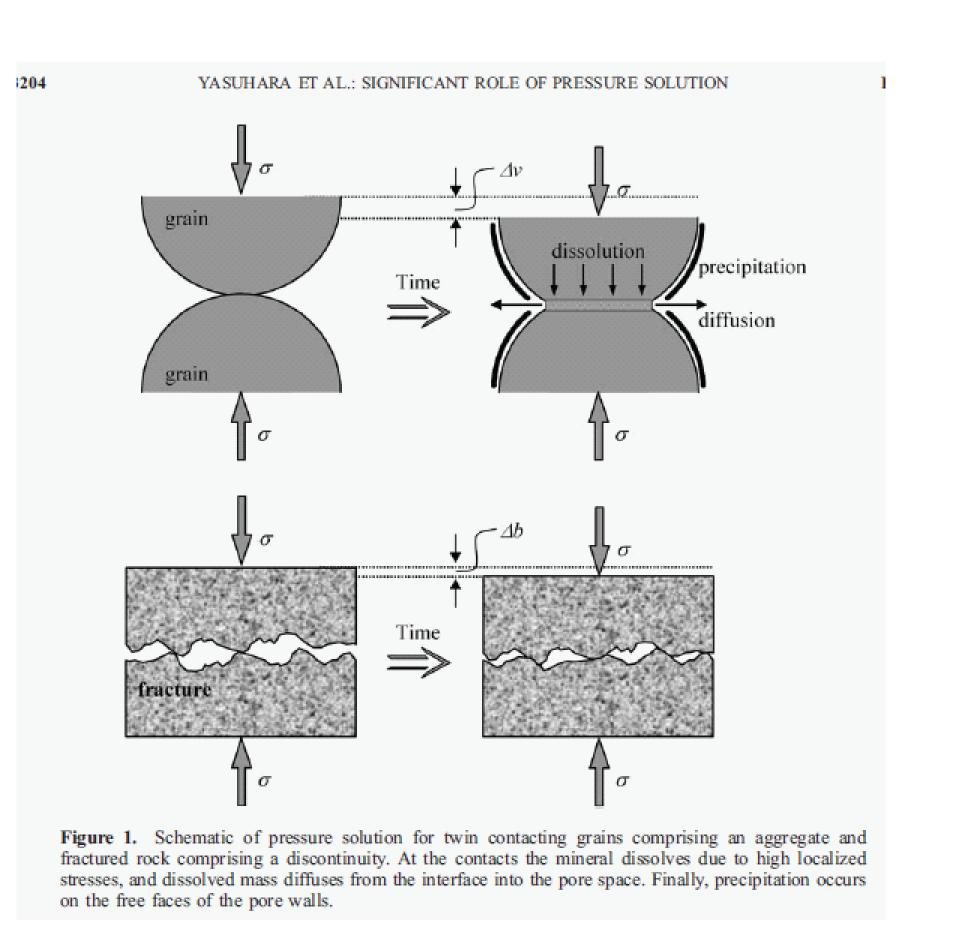
Fig. 6: Conceptual model for permeability reduction due to reactive flow under a load, explaining the observations in Fig. 5. Healing of the fracture is due to pressure solution, causing viscous compaction (Yasuhara et al., 2004).
