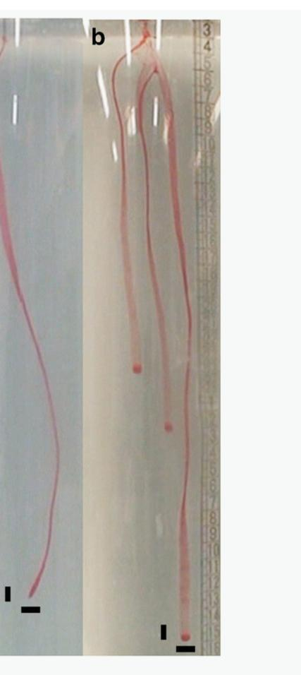
Examples of the trajectory of the injected fluid showing (a) "III. meanderi D)"  $(C = 0.2 \text{ wt.\%} \Delta \rho = 299 \text{ kg m}^{-3})$ , and (b) "IV, bifurcate (2D)" (C = 0.1 wt.%) $= 299 \text{ kg} \text{ m}^{-3}$ ). Scale bars are 10 mm. Injection point can be seen at the top. In (a), he apparent thickness of the crack changes as it descends because of the twisting of the
