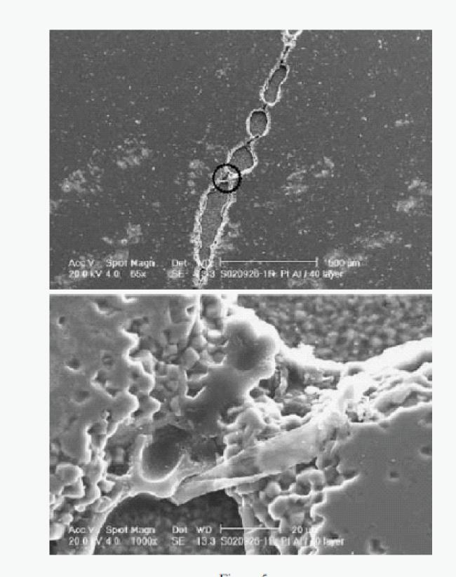
SEM of fracture post test, showing locations of welded fracture [courtesy A.B. Polak].
