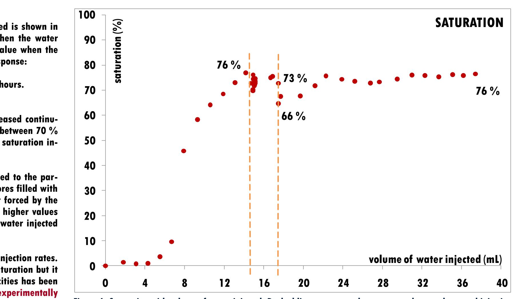
Figure 6. Saturation with volume of water injected. Dashed lines represent the moments when we decreased injection rate, at 14.6 mL of volume of water injected, and when we stopped and restarted injection, at 17.5 mL.
