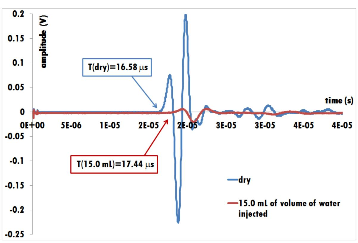
Figure 1. Waveforms for the P-waves picked during our experiment: before injection (blue line) and after injecting 15.0 mL of volume of water (red line). Note the decrease on waveamplitude and an increase on the P-wave arrival time with the presence of water.
