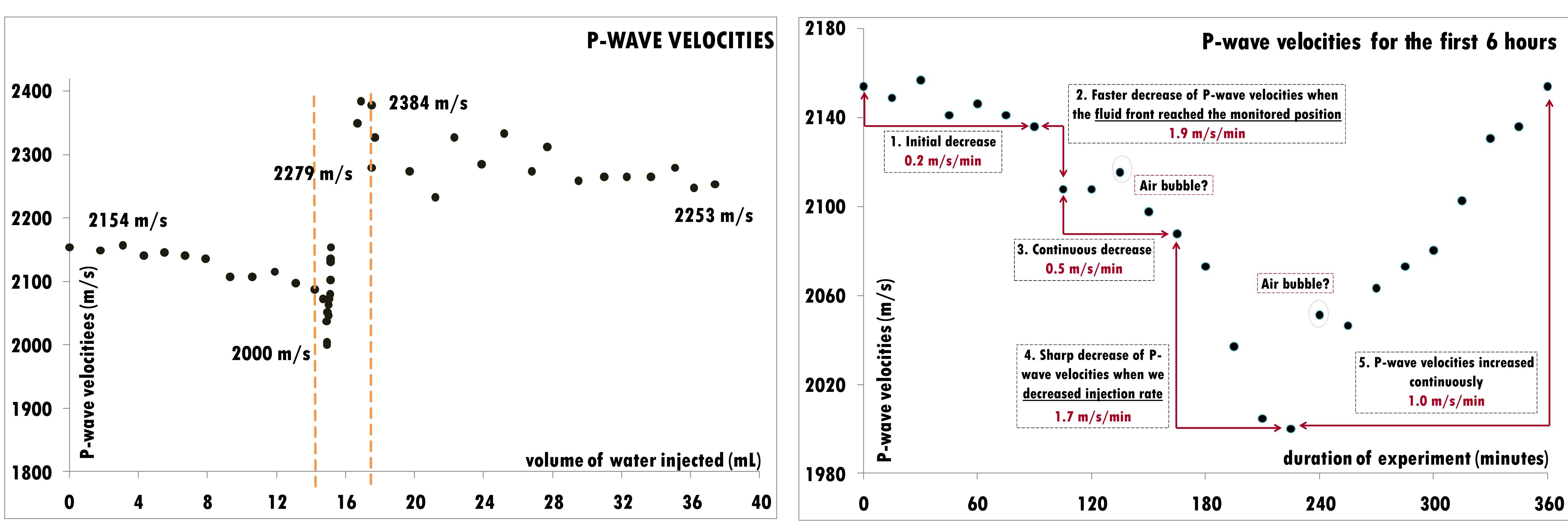
Figure 4. P-wave velocities with volume of water injected. Dashed lines represent the moments when we decreased injection rate, at 14.6 mL of volume of water injected, and when we stopped injection and restarted, at 17.5 mL. Note the sharp decrease followed by an increase of 384 m/s after decreasing the injection rate from 5 mL/h to 0.1 mL/h and a striking oscillation effect after we restarted injection at 5 mL/h.
