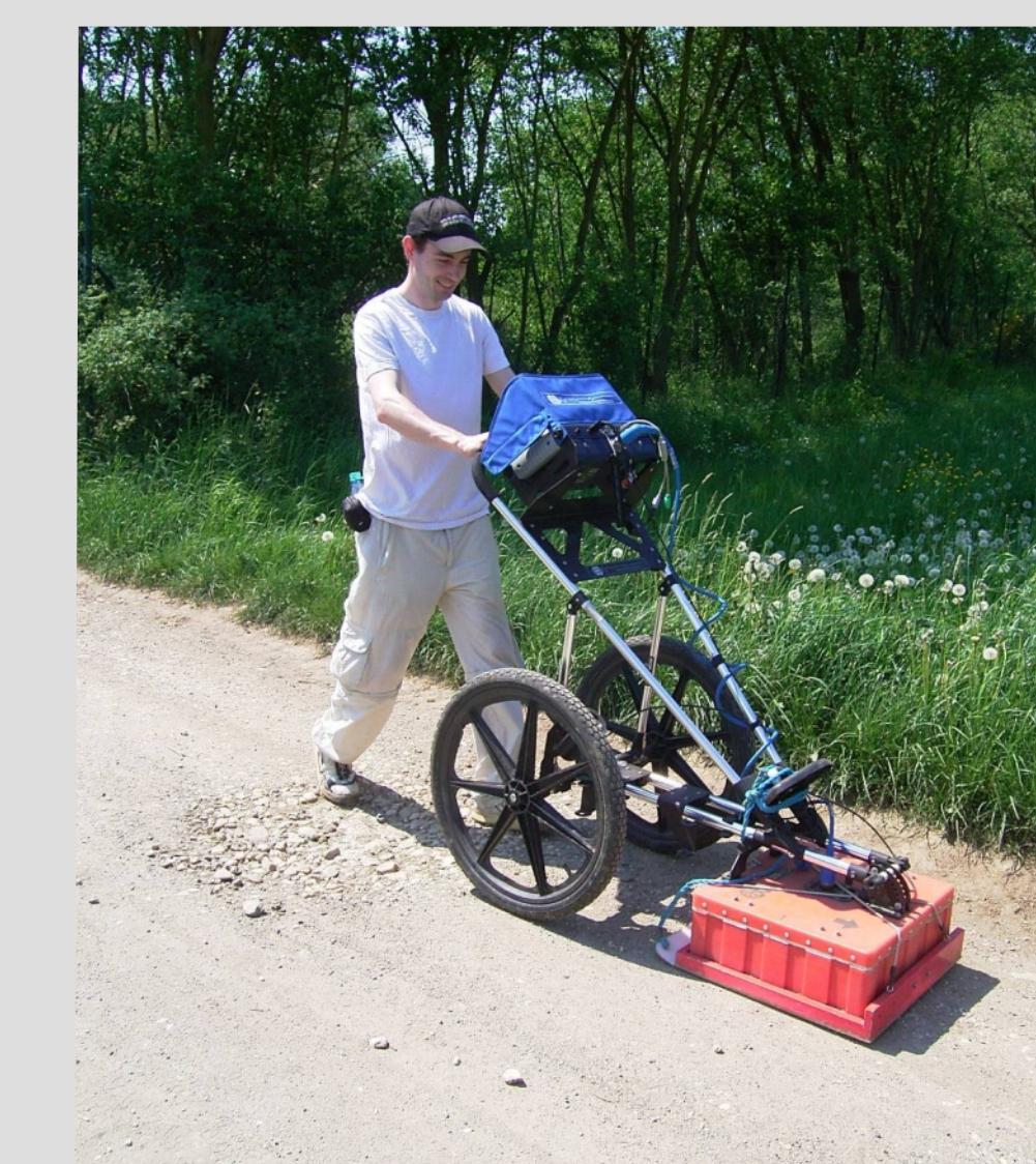
Figure 4: GPR measurements (270 MHz).
