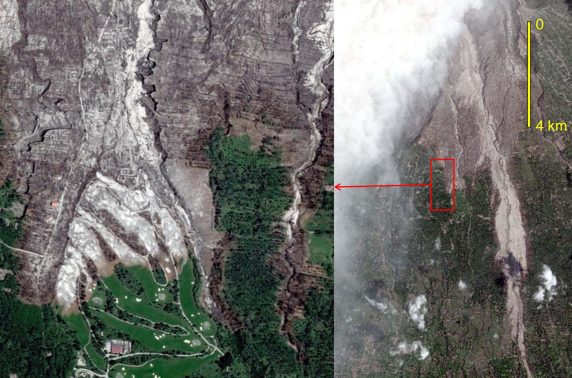
Volume of pyroclastic debris likely to be removed by rain in valleys (in excess of  $100 \times 10^6$  cubic-meters) much higher than those calculated after more conventional eruptions (less than  $10 \times 10^6$  cubic-meters);
