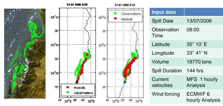
The position of the oil slicks predicted by B) **CYCOFOS-MEDSLIK** C) **MFS-MEDSLIK**, corresponding to July 23 8:00 GMT compared with A) the slick observed by MODIS ACQUA (green)
