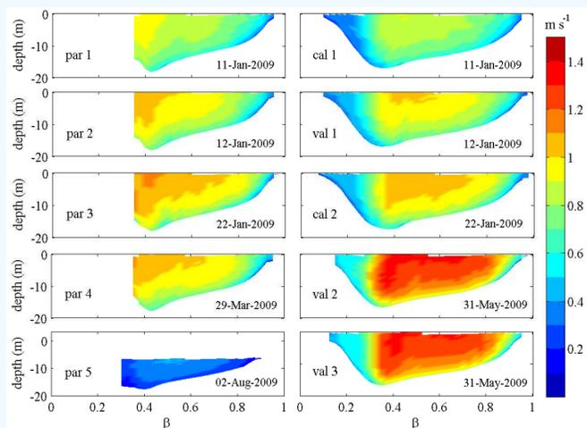
Streamwise velocity during boat-mounted ADCP campaign.
