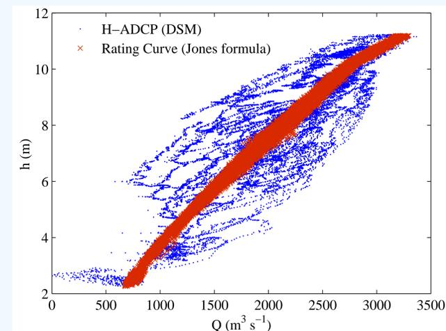
Stage and discharge from rating curve and from H-ADCP data.
