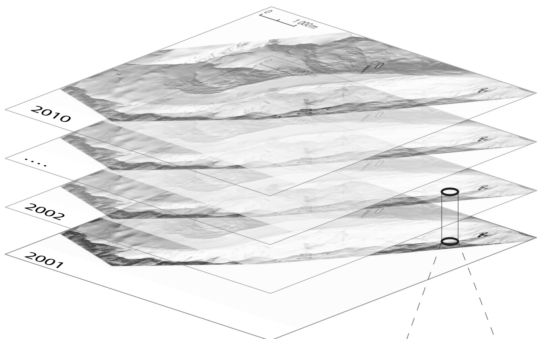
This poster shows the ability of airborne LiDAR techniques to detect, map and quantify specific geo-morphological entities in selected high alpine catchments. Since 2001 airborne LiDAR measurements have been carried out regularly in the Hinter-eisferner region (Ötztal Alps, Tyrol, Austria). This results in a worldwide unique consistent data record assembling 18 LiDAR campaigns. The focus is on glaciated and recently deglaciated (periglacial) terrain and in particular on:
