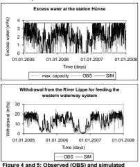
(SIM) excess water at Hünxe (top) and water withdrawal from the River Lippe (bottom)
