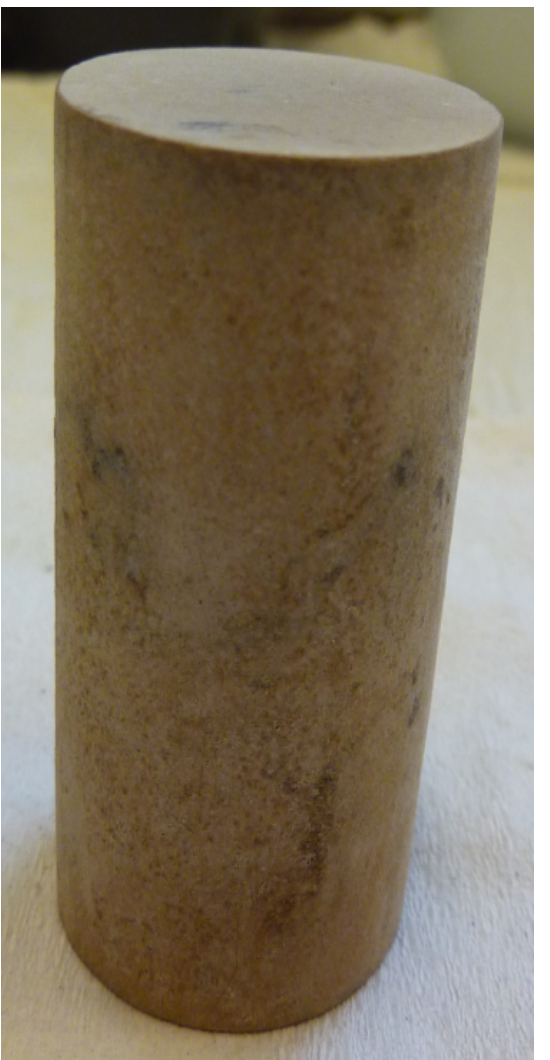
Cement sample aged during 14 days. (L=50mm, Ø=25mm)
