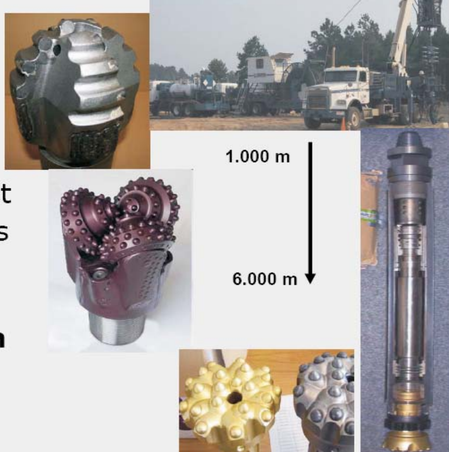
Pic. 1: Summary of old and new drilling tools like PCD / tricone bits as well as new DTH fluid hammer tooling
