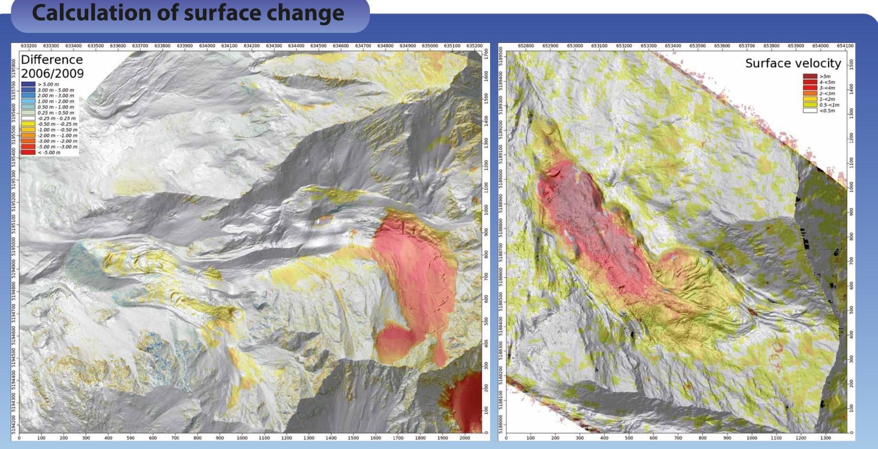
Digital elevation models of the years 2006 and 2009, derived from airborne laser scanning point clouds, were used to calculate vertical differences in the surface of the rockglaciers. Hillshades were used to determine surface velocities.
