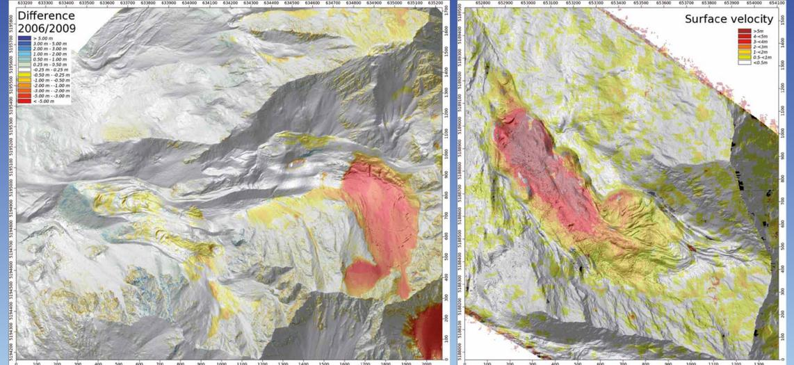
Digital elevation models of the years 2006 and 2009, derived from airborne laser scanning point clouds, were used to calculate vertical differences in the surface of the rockglaciers. Hillshades were used to determine surface velocities.
