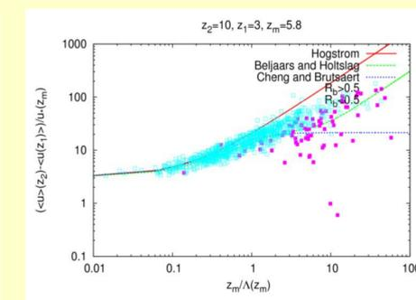
Figure 5. : Velocity difference normalised with  $u^*$  as function of  $z/\Lambda$ . Open squares: data with  $Rb < 0.5$  (moderately stable), full squares: data with  $Rb > 0.5$ .
