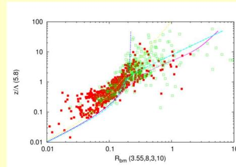
Figure 3.  $z/\Lambda$  vs.  $Rb(3.55, 8, 3, 10)$  from the observations. Here Sorbjan et al. (2010), Eq. 24 is used. Full squares: SBL with TKE decreasing with height; open squares: TKE increasing with height.
