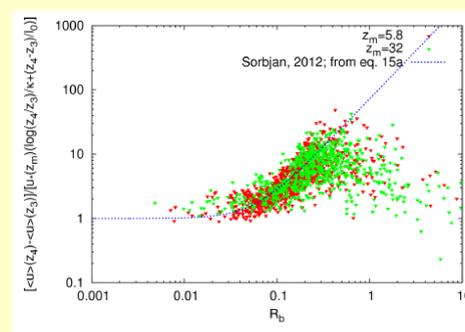
Figure 4. Velocity difference normalised according to Eq.8 as function of bulk Richardson number.
