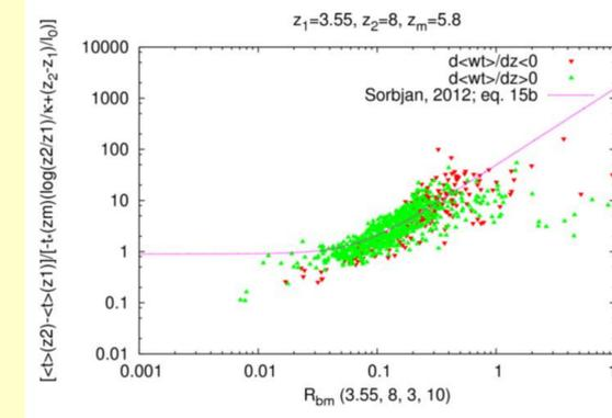
Figure 7. Temperature difference normalised according to Sorbjan formulation, as function of the bulk Richardson number.
