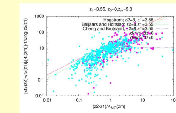
Figure 6. : Temperature difference normalised over  $t^*$  as function of  $z/\Lambda$ .
