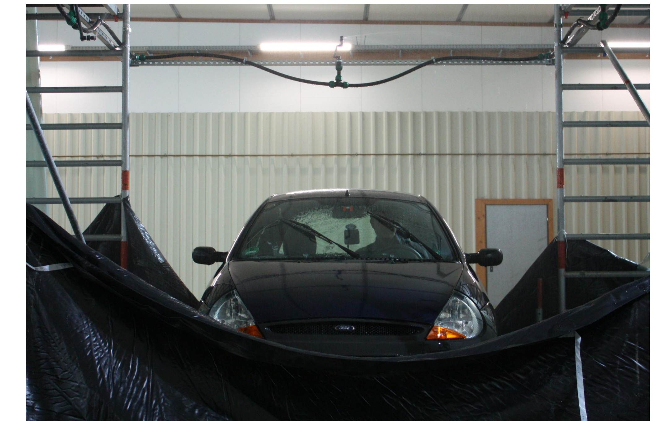
Fig. 5: cars with different wiper systems are being investigated under different rain intensities produced by a sprinkler irrigation system in laboratory. By changing the nozzles and the pressure on the nozzles different intensities are adjusted. The produced rainfalls, measured by conventional rain gauges, is recorded in a PC and analysed against wiper frequencies, afterwards.
