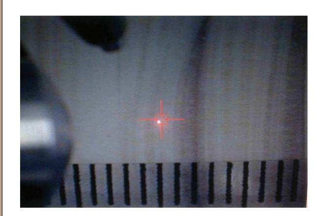
FIGURE 2: A) Brüker ARTAX µ-XRF system, scanning stalagmite in lab. B) Close-up view of ARTAX during scanning. Tube is attached to an x-y-z stage that can be programmed to account for a slanted stalagmite surface. C) Digital onboard camera view of scanning mode. Laser pointer indicates location of XRF beam during analysis. If desired, a digital snapshot of each analysis point can be collected.
