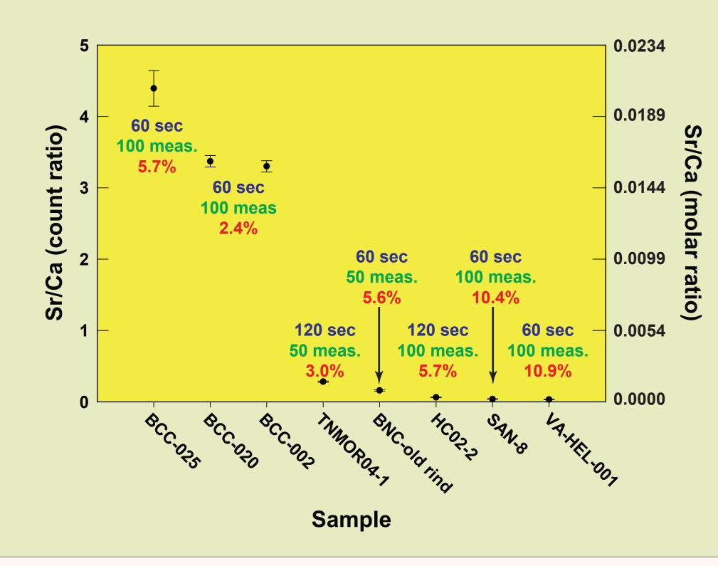
FIGURE 4: Demonstration of the reproducibility  $(1\sigma)$  of the same point, given different stalagmites with different Sr/Ca ratios.
