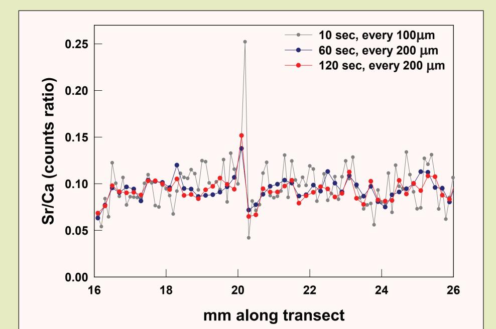
FIGURE 3: Demonstration of effects of count time on reproducibility of Sr/Ca record. The same transect was analyzed at 10, 60, and 120 seconds. Note how, despite the "jumpiness" of the record, the transect from the 10-sec count time largely reproduces the results obtained from transects with longer count times.
