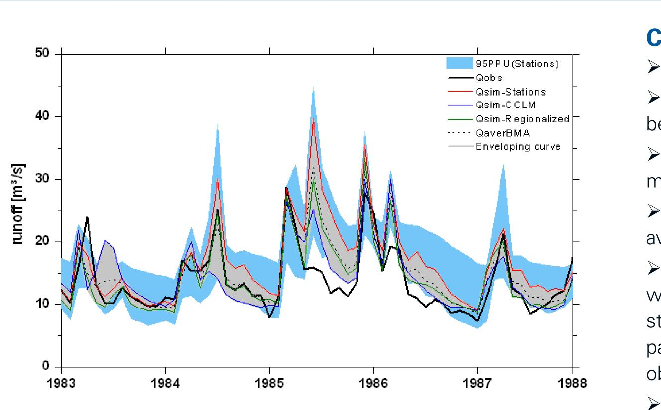
Fig. 4: Observed and modeled hydrographs of three models, their enveloping curve, BMA and the uncertainty band of the model *Stations* (95PPU) for the calibration period.
