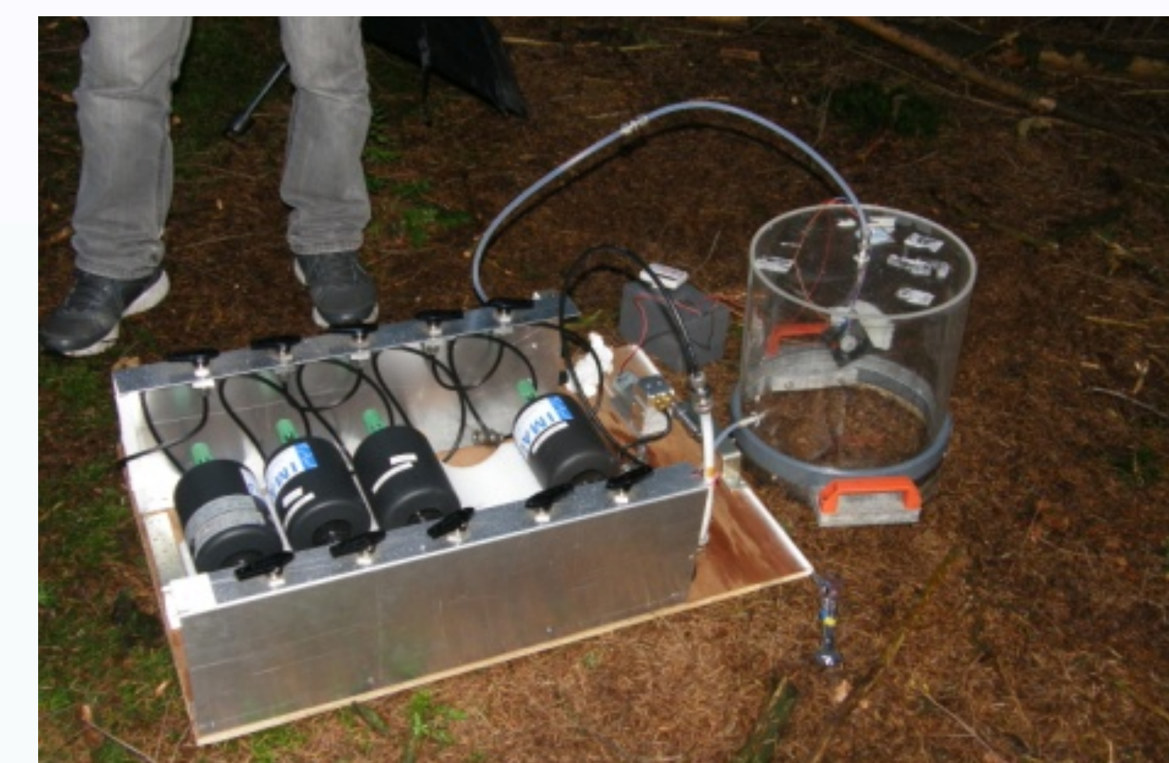
Fig. 1b Flask sampler and soil chamber
