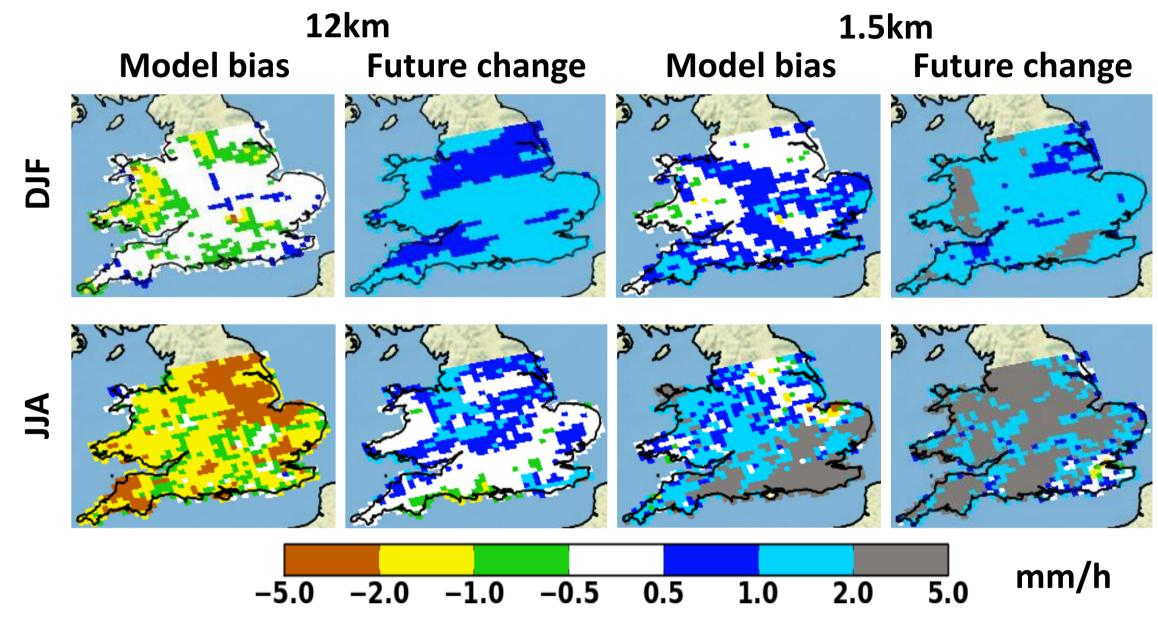
Fig 4. Model biases and future changes in heavy rainfall at the hourly timescale in the 12km (left) and 1.5km (right) models, for winter (top) and summer (bottom)
