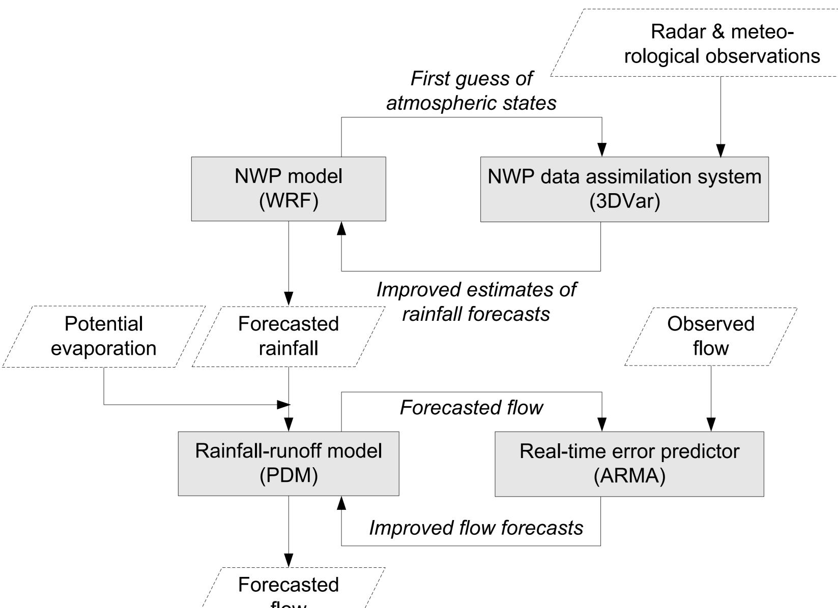
Fig. 1 Components of the real-time flood forecasting system with inputs and outputs framed by dashed lines
